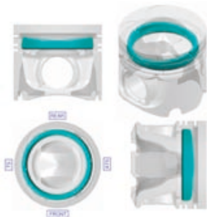
Fig. 10: Piston 1 (Gallery w/ Variable Cross Sections)
