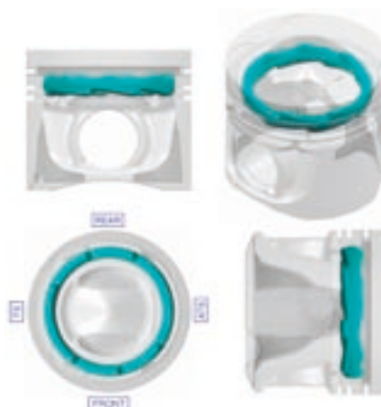
Fig. 12: Piston 3 (with Dual Arm Cooling Gallery)
