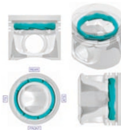
Fig.11: Piston 2 (Gallery with Stepped Chamber Segments, DynamiKS™)
