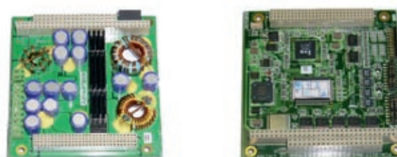
Figure 7: Advantech Power supply and PCI to ISA boards (source: Advantech Corp.)
