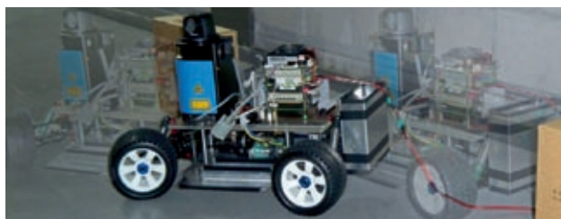
Figure 1: The scaled 1:8 Robocar during the parallel parking procedure (source: R. Gall)
