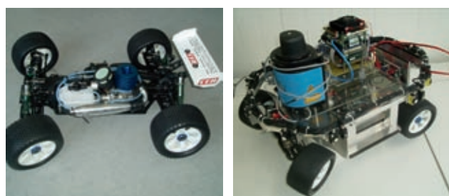
Figure 4: A comparison between the original scaled vehicle and the robocar. (source: R. Gall)
