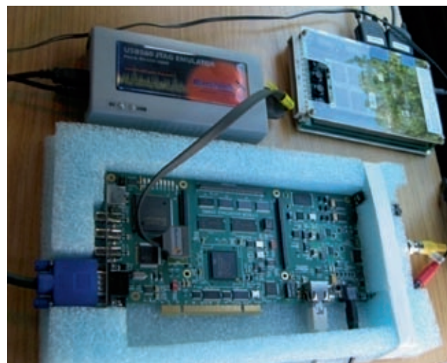
Figure 10: The Texas Instruments board and Blackhawk JTAG Emulator. (source: R. Gall)
