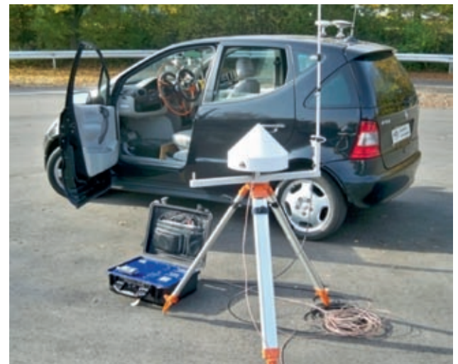
Figure 3: The full scaled A Klasse driving robot with the DGPS station. (source: R. Gall)
