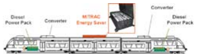
Fig. 6: Principle scheme of a diesel electric vehicle equipped with MITRAC Energy Saver
