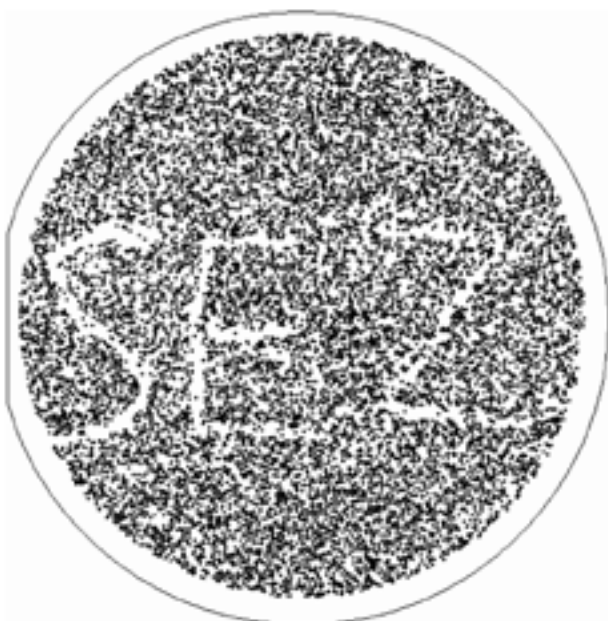
Figure 2: Removal of van-der-Waals bonded \text{Si}_3\text{N}_4 particles by a focused water stream (> 400 nm, Surfscan 7200).
