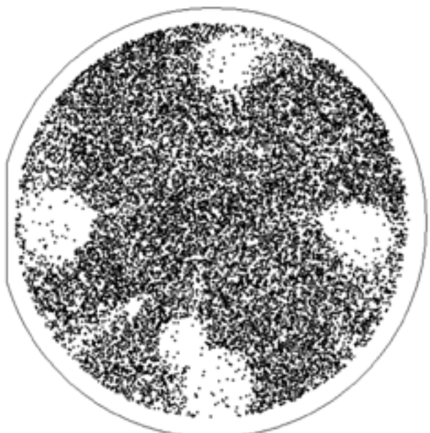
Figure 4: Removal of van-der-Waals bonded \text{Si}_3\text{N}_4 particles by colloidal silica Ludox TMA (> 400 nm, Surfscan 7200).
