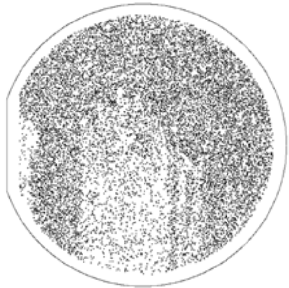
Figure 3: Removal of van-der-Waals bonded \text{Si}_3\text{N}_4 particles by polysilicates (> 400 nm, Surfscan 6220).
