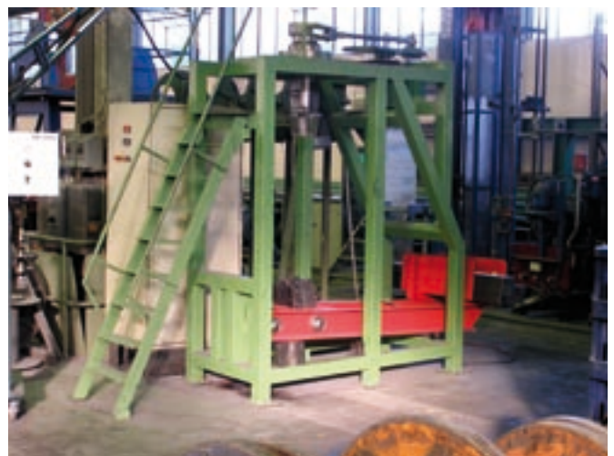
Fig. 2: Test rig for investigation of torque cycle fatigue of wire ropes
