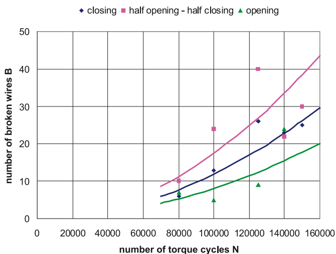
Fig. 5: Influence of number of torque cycles to number of broken wires.
