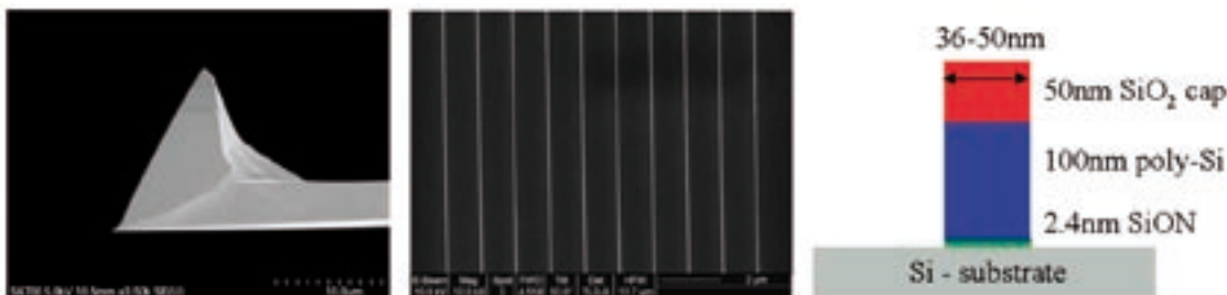
Figure 3: SEM picture of the type of AFM tip used for the collapsing experiments (left side) & “ASAP Line” structures under investigation as SEM picture and the principle design of the patterns on the right side
